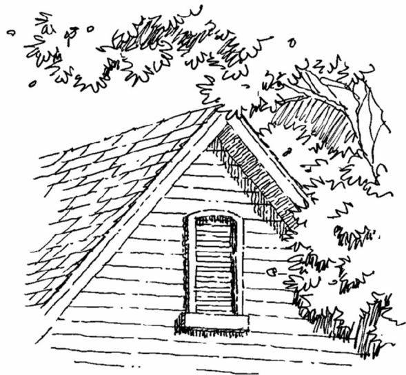
Gable end vent
